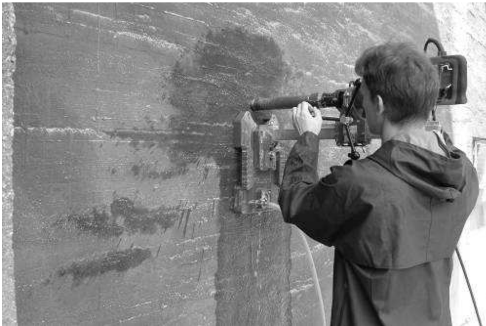
Photo 2.5: Taking samples by drilling
