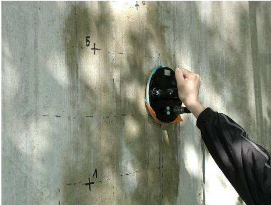
Photo 2.4: Measuring corrosion rate
