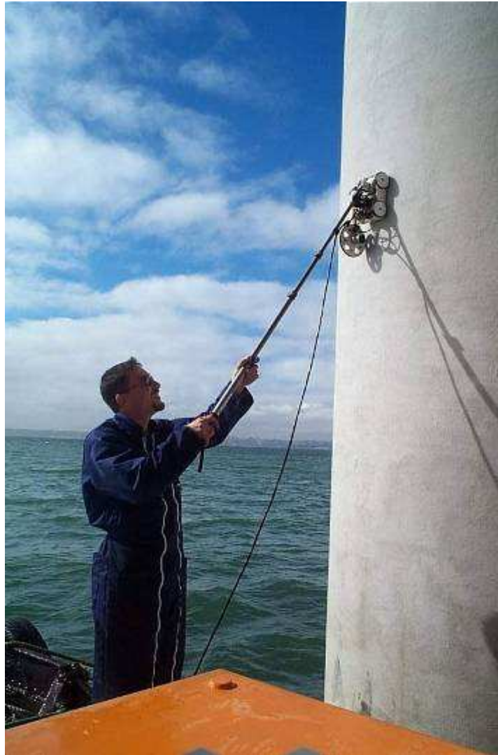
Photo 2.1: Locating reinforcements with a radar
