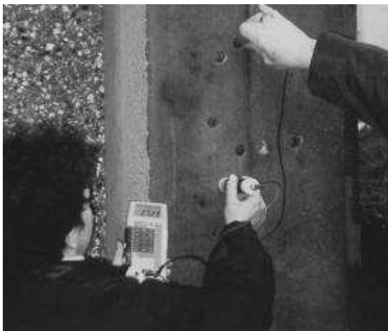
Photo 2.2: Measuring half-cell potential
