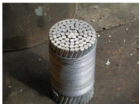
Photo 11 : Fabrication des haubans TMC / Multi-layer strand cables manufacturing
