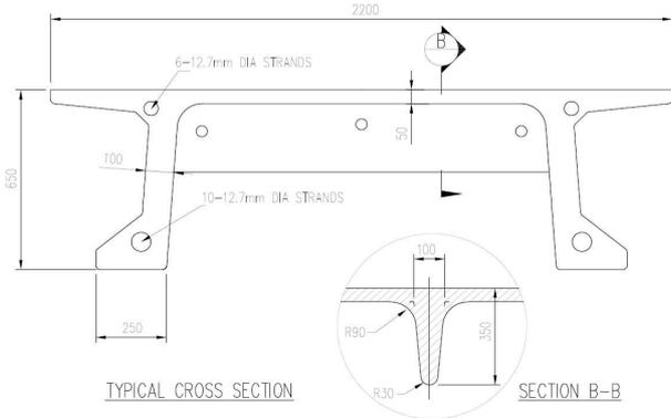
b. Cross section of UHPC beam element
