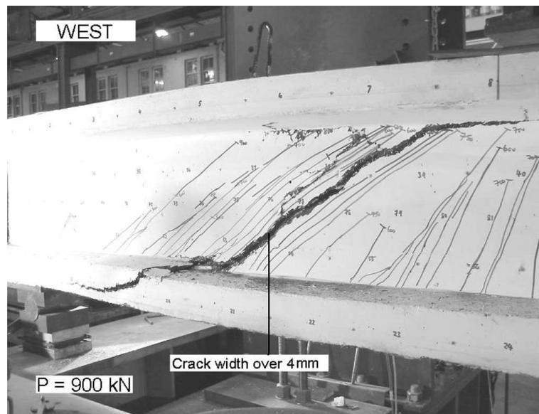
Fig. 1 UHPC beam No. 2 after shear failure
