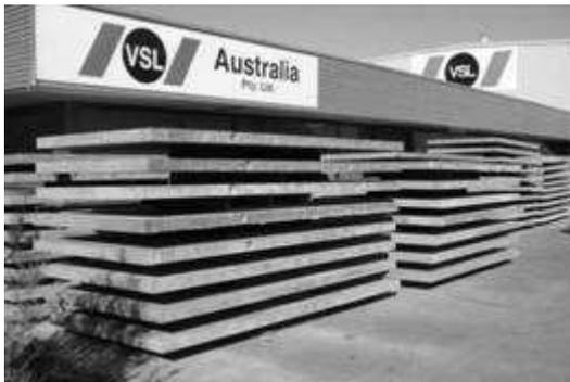
a. UHPC blast resisting panels
