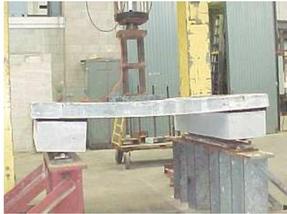
b. Test slab at a simulated wheel load of
