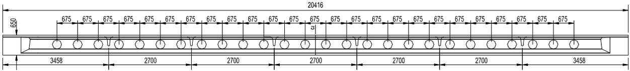
a. Typical elevation of a 20.4 m  $\pi$ -shaped UHPC (Ductal<sup>®</sup>) beam
