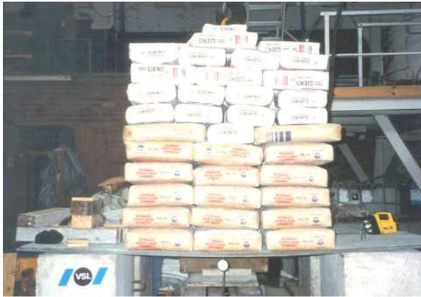
a. 25mm thick formwork slab, span 1.3m
