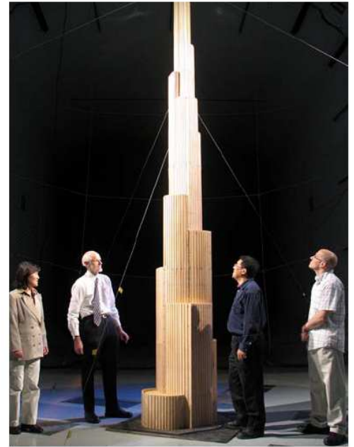
b) Rigid Pressure Tapped Model of Top Portion at 1:50 Scale
