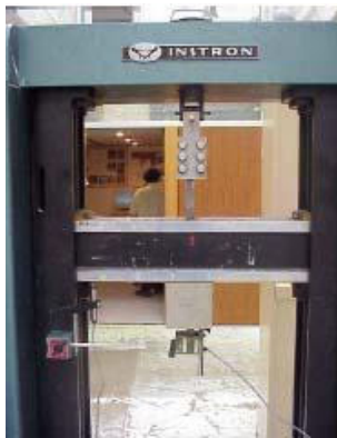
Figure 131 : Essai pull-out (LMT)
