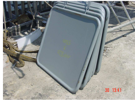
Photo 23 : Flat jacks with unusual dimensions: 810 mm x 890 mm (maximum pressure of 15 MPa) Vérins plats de dimensions inhabituelles de 810 mm x 890 mm (pression maximum 150 bars).
