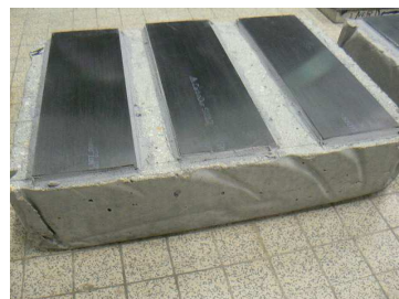
Fig. 6. Concrete specimen reinforced with bonded CFRP plates (3 layers)
