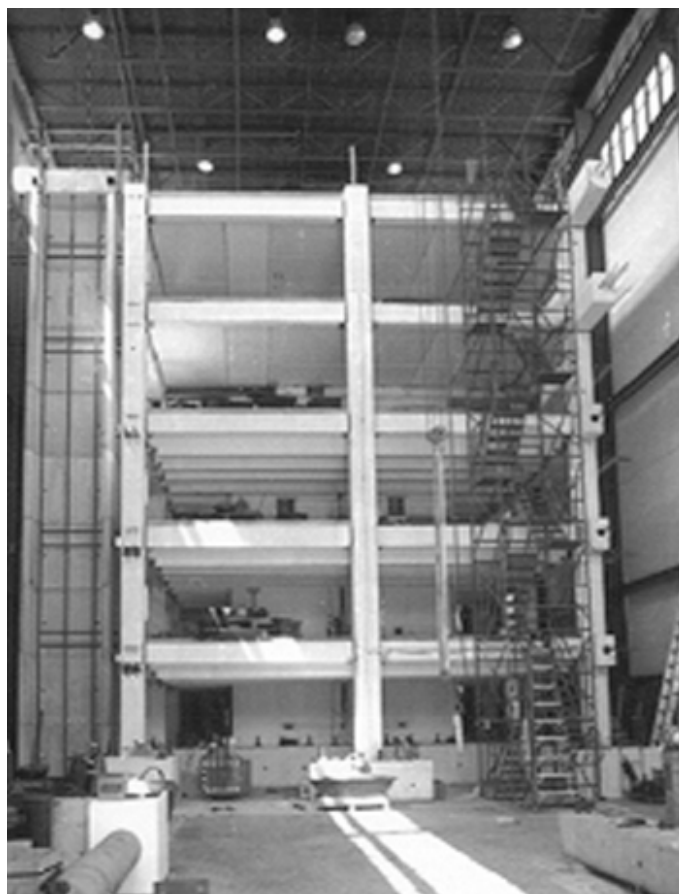
Fig. 5-52: Overall view of the five-storey building tested under the PRESSS programme [Priestley, (1999)]
