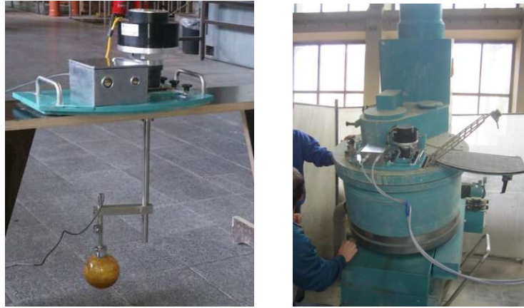
Figure 2. Concrete Rheometer RheoCT – application in a laboratory concrete mixer
