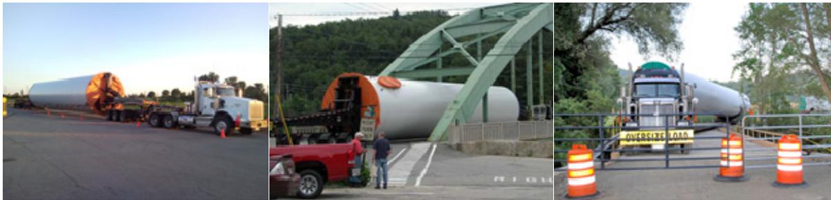
Figure 1: Transportation of steel tower segments and associated challenges [1]
