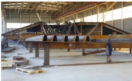
Work on the frames in the workshop: main box girder of the lift span and outriggers supporting the sidewalks
