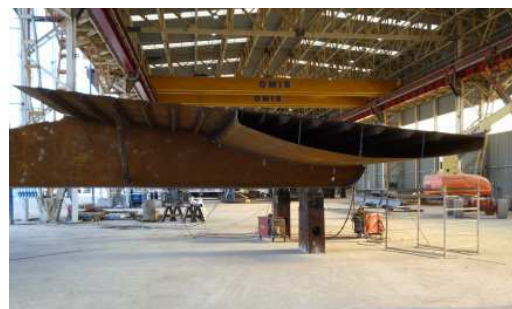
Work on the frames in the workshop: main box girder of the lift span and outriggers supporting the sidewalks
