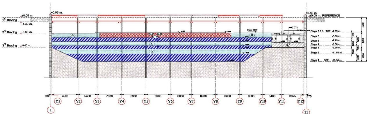
Fig.5. Casting sequence of mat foundation. Source Bouygues – Thai)
