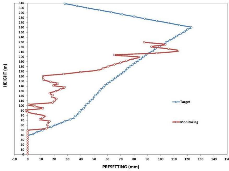
Fig.13. Target and monitoring pre-setting (Source Bouygues-Thai)
