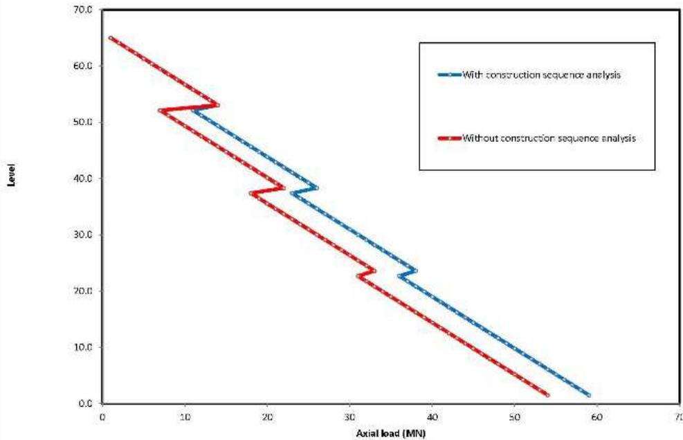
Fig.8. Effect of a construction sequence in column loads. (Source Bouygues-Thai)
