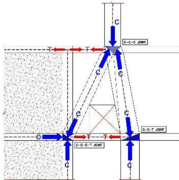
Fig.9. Strut-and-tie truss model for the level 19-20 outrigger.(Source Bouygues-Thai)
