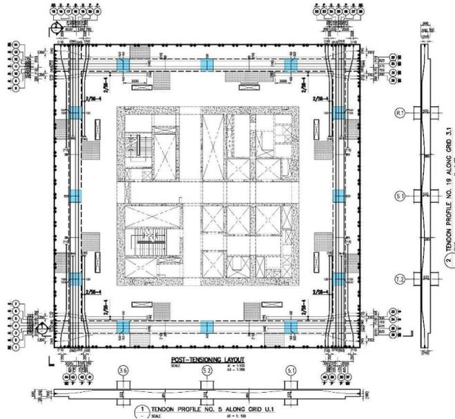
Fig.11. Post-tensioning layout (Source Bouygues-Thai)
