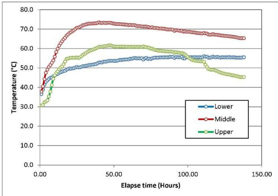
Fig.4. Concrete temperature monitoring. (Source Bouygues – Thai)
