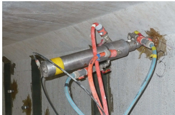
Figure 12 : corrosion inhibitor ultrasonic transducer
