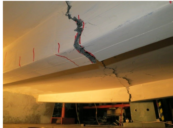
Figure 8: Bending failure of the ribs
