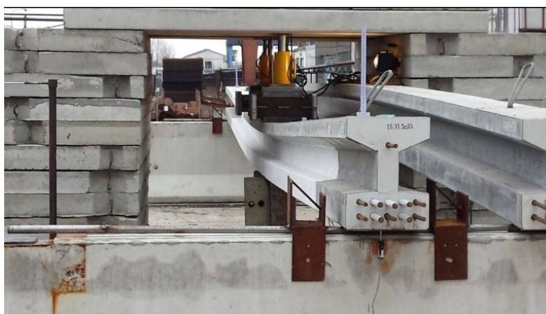
Figure 1: Deflection of the pretensioned UHPC beam during testing, an unloaded UHPC beam with upwards camber due to prestressing is nearby
