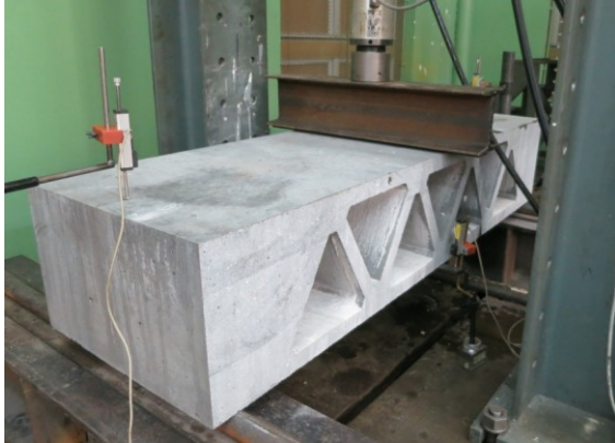
Figure 2: Arrangement of the 3 point bending test
