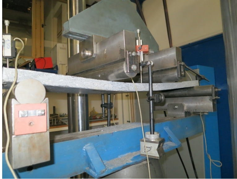
Figure 8: 4-point bending test of the slab strip
