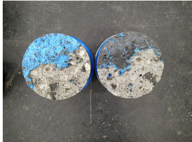
Figure 8: Specimen BA1 fractured at the UHPFRC – concrete interface
