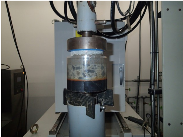
Figure 6: Application of tensile fatigue force to specimen immersed in water
