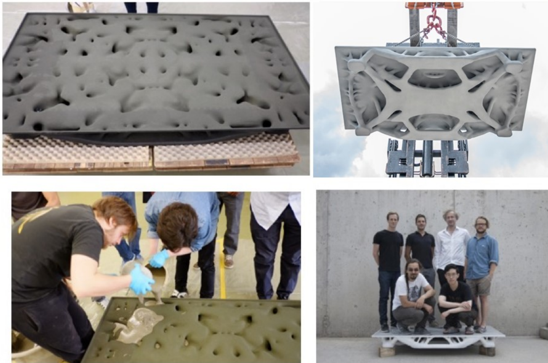
Figure 7: Top view of element, pre infill (top left); Bottom view of element, post infill (top right); Infill process (bottom left); Final element after casting (bottom right)
