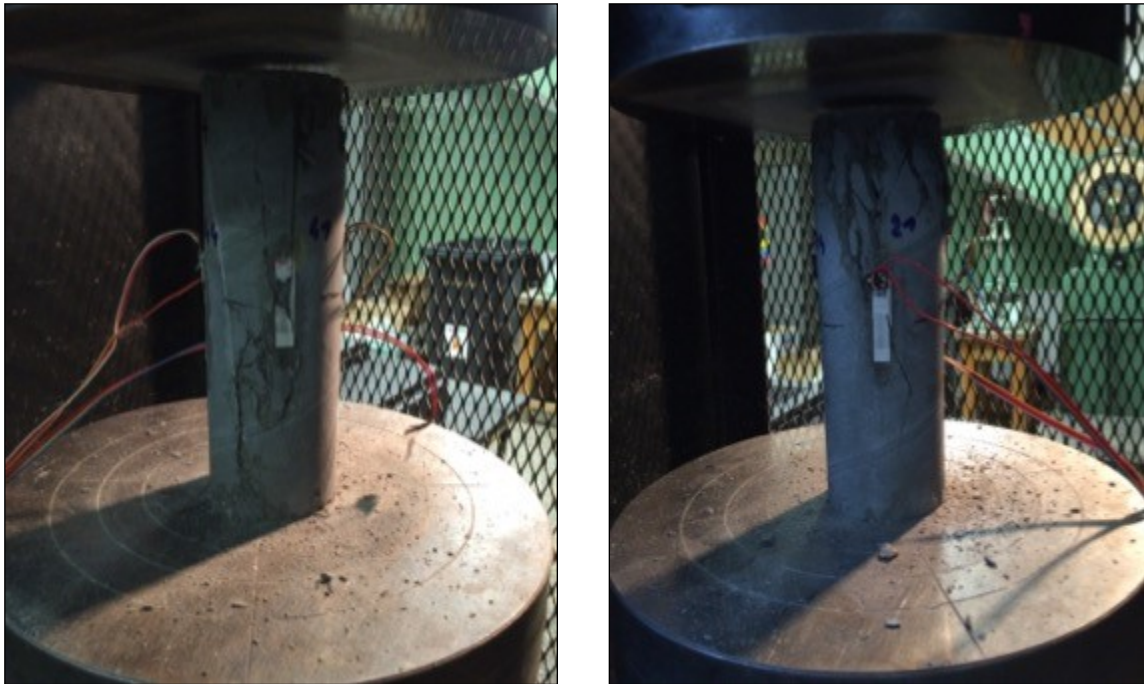
Figure 4: Typical damage pattern – specimens after static tests
