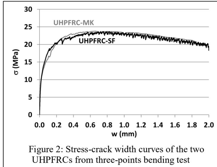
Figure 2: Stress-crack width curves of the two UHPFRCs from three-points bending test
