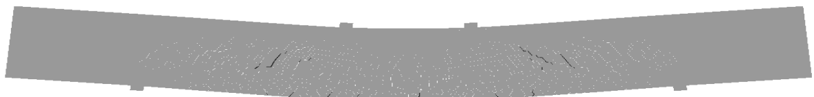
Figure 7: Example of cracking process of the reinforced beam loaded in shear
