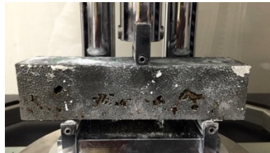
Photo 2: Sample with steel fibers showing cavities
