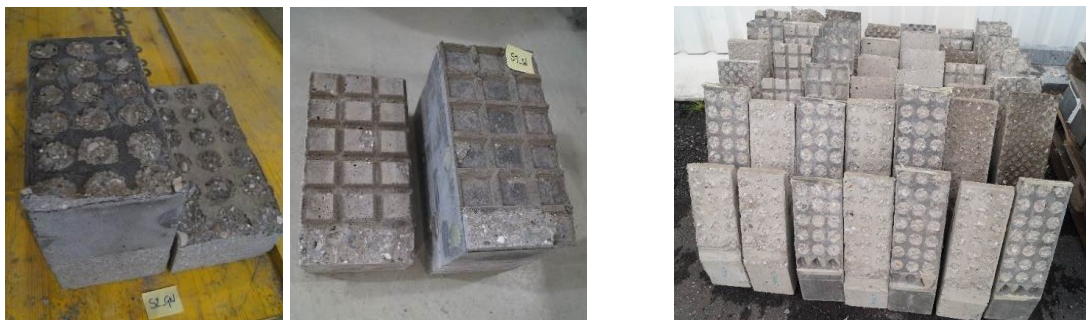
Figure 8: Interface profiles after push-out (left) and slant shear tests (right)
