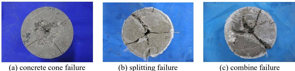
Figure 4: Three concrete failure modes in the pure-tensile tests.
