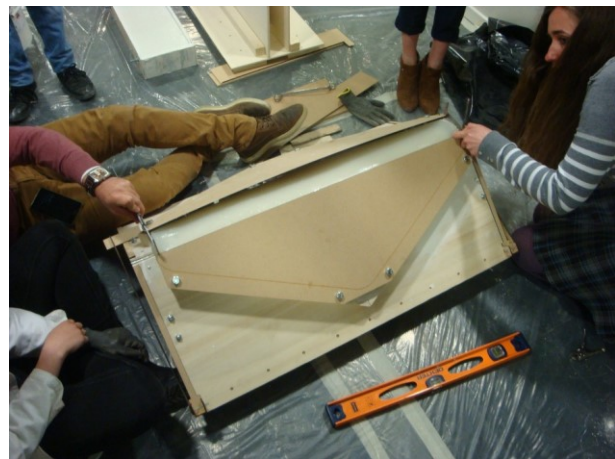
Figure 4: Flexible mould (images Raphaël Fabbri)
