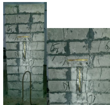
(b) Failure mode of UHPM masonry short column
