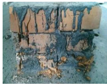
(a) Failure mode of CM masonry columns (b) Failure mode of UHPM masonry columns
