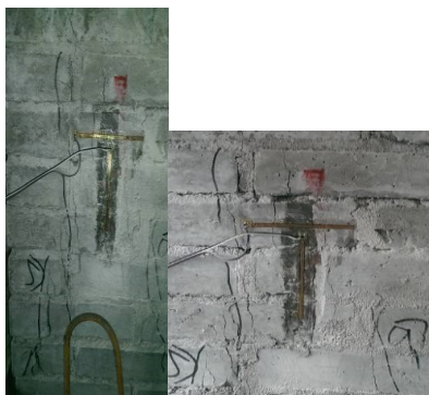
(a) Failure mode of CM masonry short column
