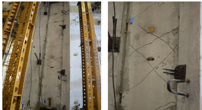
Figure 5: Cracking of the two HSC connecting panels after completion of operational torsional loading
