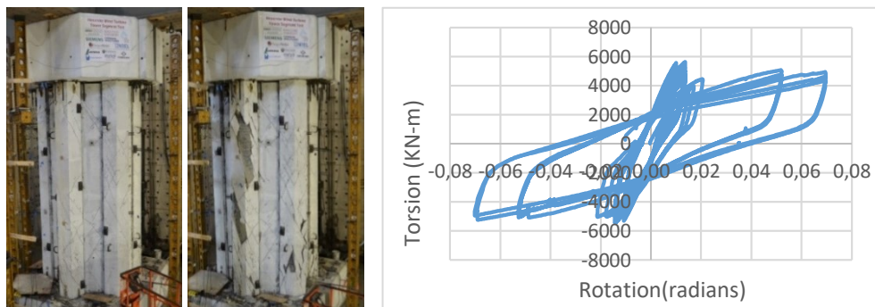
Figure 8: Large displacement damage (left) and response (right) of test unit
