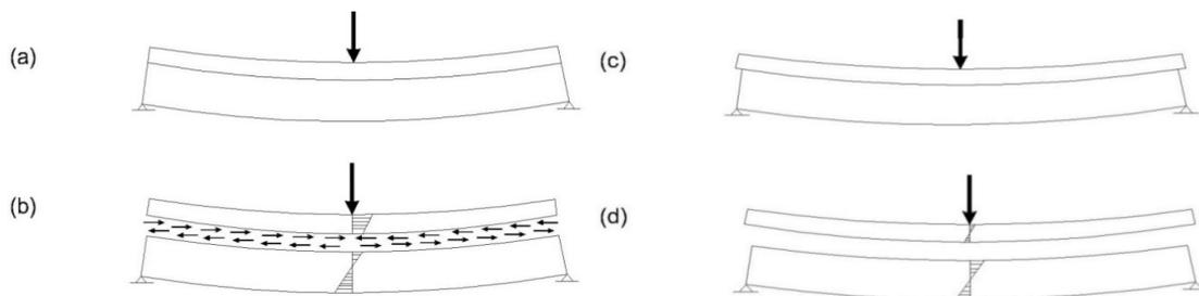
Figure 1: Simply supported beam: (a) composite beam, (b) shear stresses at the interface, (c) non-composite beam, and (d) horizontal shear slip. Adapted from reference [4]
