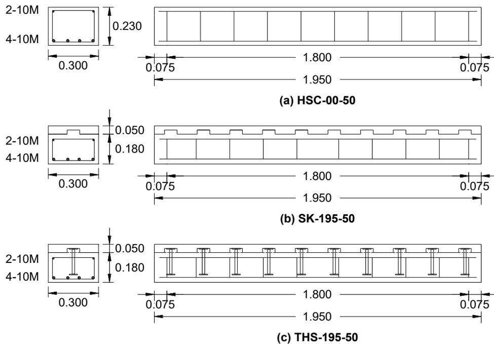
Figure 2: Details of test specimen (all dimensions are in meters)
