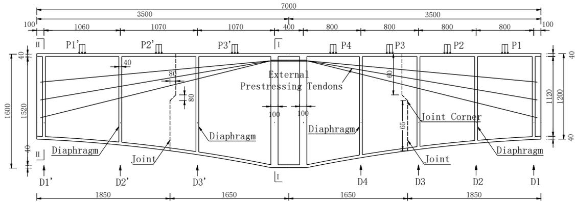
(a) elevation view (unit: mm)
