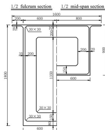
Figure 2: Main cross sections of LPUBG (unit: cm)
