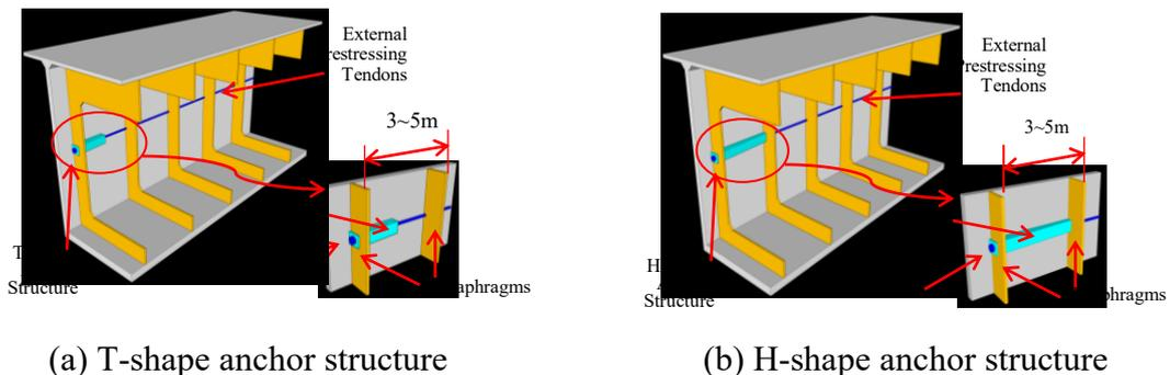
Figure 9: Schematic diagram of anchor structure in LPUBG
