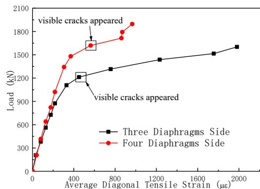
Figure 7: Load-strain curve of the web joint
