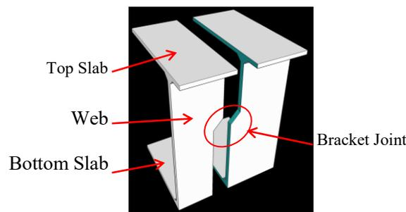
Figure 6: Schematic diagram of bracket joint
