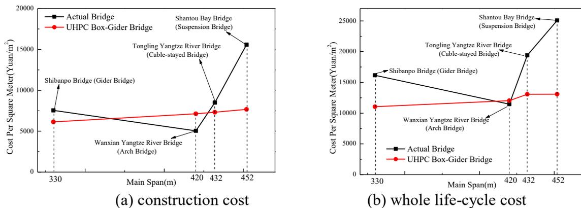
Figure 8: Cost comparison between actual bridges and LPUBG bridges
