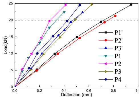
Figure 4: Load-deflection curve of top slabs
