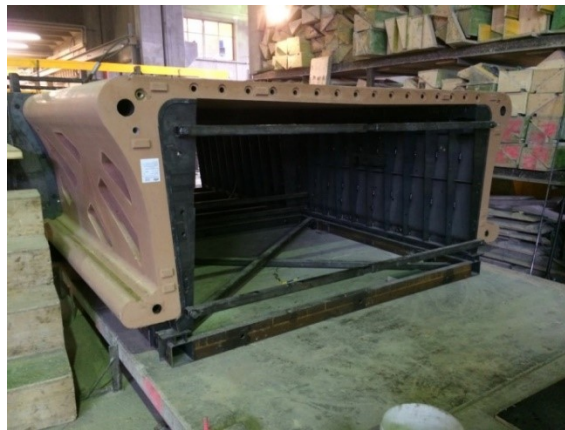
Figure 4: A segment after formwork removal, with its wind bracing system
