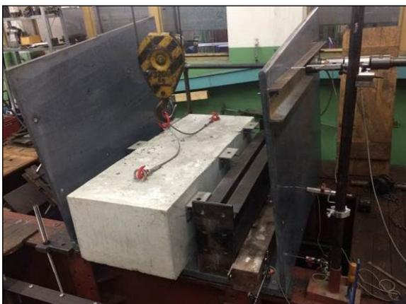
Figure 7: Test of load bearing capacity of the right thin wall – an inward direction
