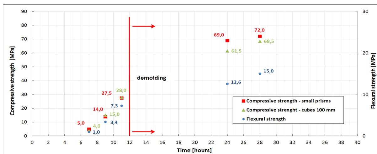
Figure 5: Development of compressive and flexural strength at first 40 hours after casting
