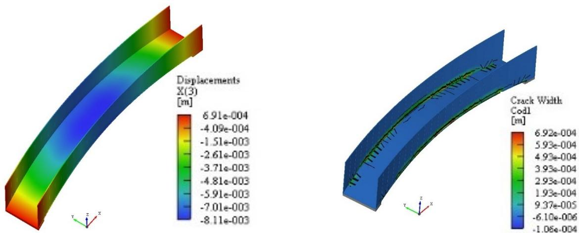
Figure 2: Vertical deflection (left) and cracks (right) of the structure before failure, the applied force of 12.6 kN /m<sup>2</sup>, the maximum deflection value -8.11 mm and the maximum crack width 0.692 mm
