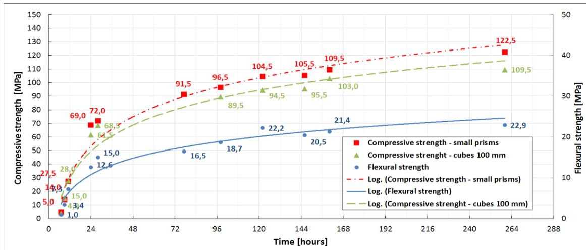
Figure 6: Development of compressive and flexural strength at first 10 days after casting
