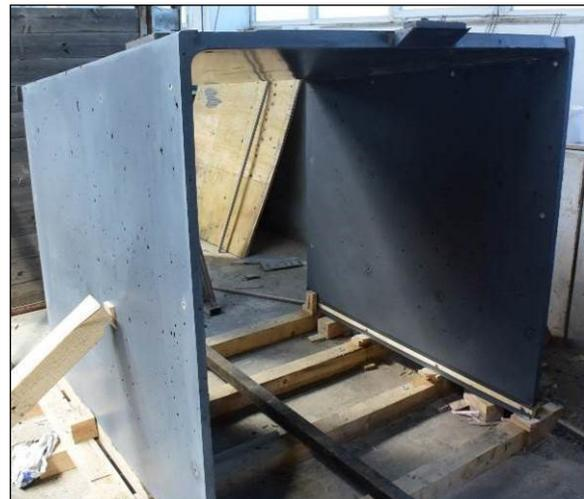
Figure 4: Preliminary mock-up after the demoulding
