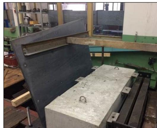
Figure 8: Test of load bearing capacity of the left thin wall – a way out direction
