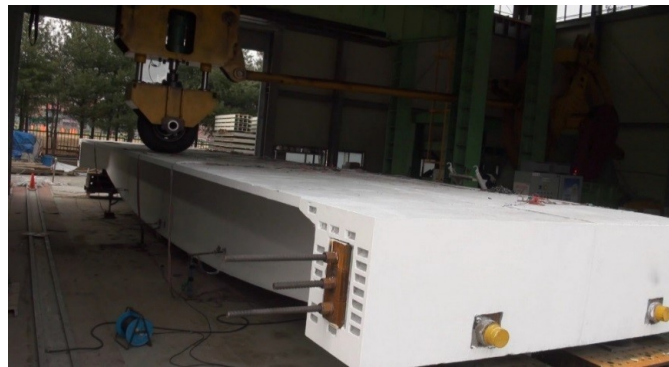
Figure 13: Rolling fatigue test of 800-m class UHPC cable-stayed bridge prototype (2011)
