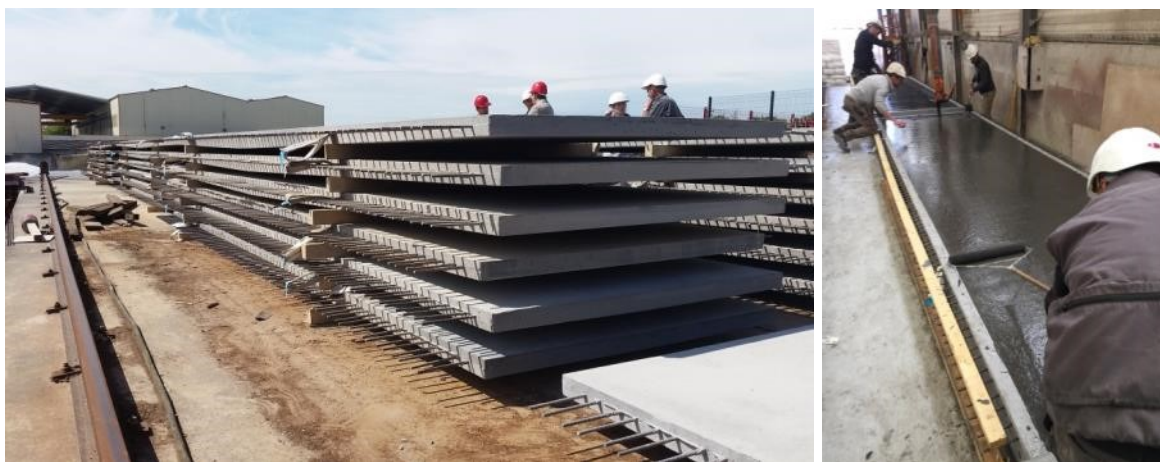
Figure 3 : Illustrations of UHPFRC slab production
