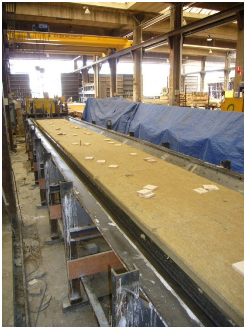
Figure 9: Formwork in the prefabrication factory Figure 10: Transportation of the \Omega -beams
