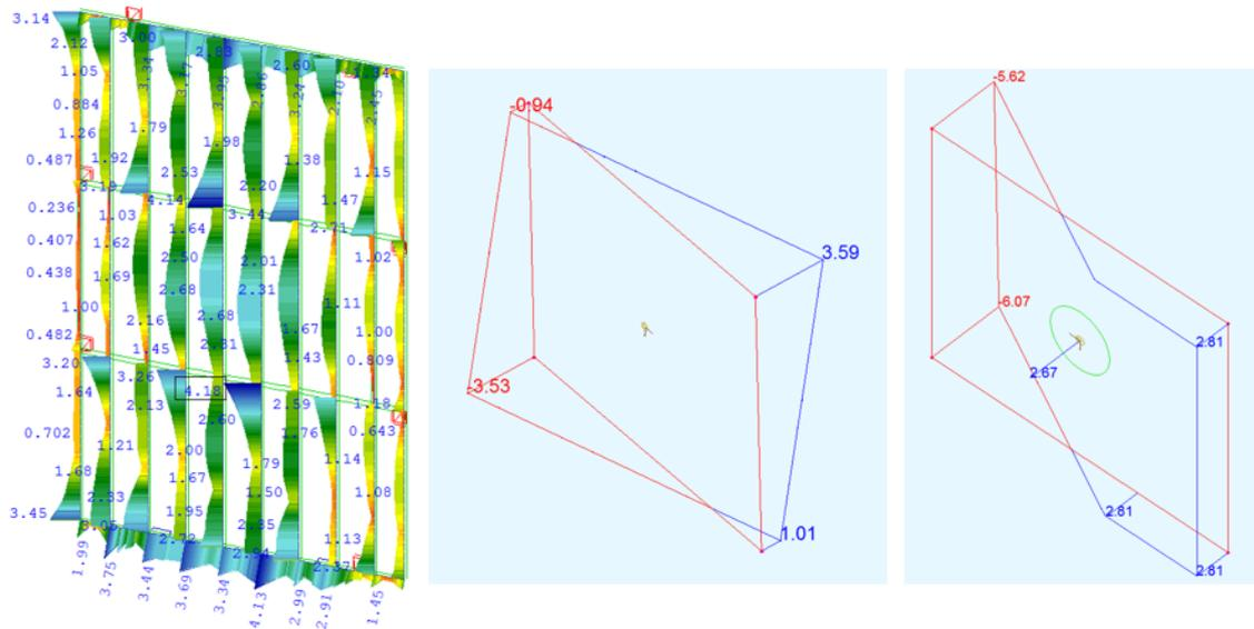
Figure 12: From left to right: Maximum tensile stress under SLS combination on unreinforced cross-section  $< 4.3\text{MPa}$  / Linear axial stress distribution of Unreinforced cross-section - SLS / Non-linear axial stress distribution of Reinforced cross-section - SLS
