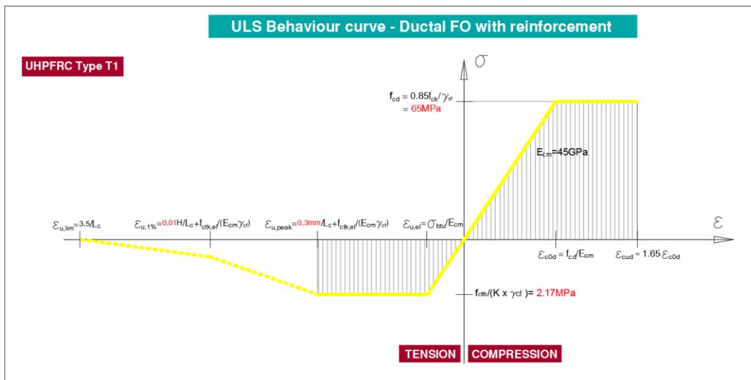
Figure 5: ULS constitutive curve – Ductal FO with reinforcement
