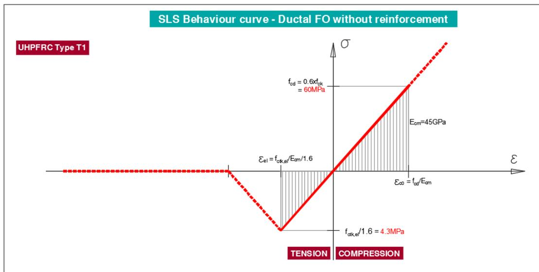
Figure 2: SLS constitutive curve – Ductal® FO without reinforcement
