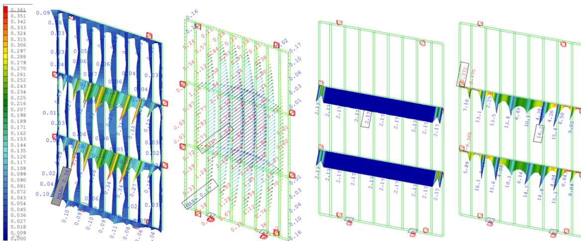
Figure 13: From left to right: Maximum elongation under SLS combination  $< 0.604\%$  / Maximum displacement under SLS combination  $< L/500=5.6\text{mm}$  / Maximum tensile stress and maximum compressive stress in reinforcement under ULS combination
