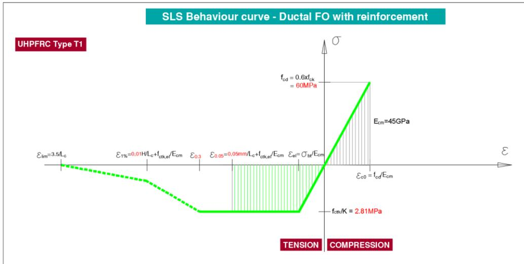
Figure 3: SLS constitutive curve – Ductal FO with reinforcement
