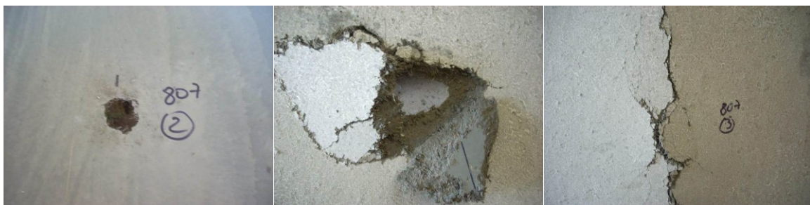
Figure 5: Failure pattern after punching tests (middle of tile)
