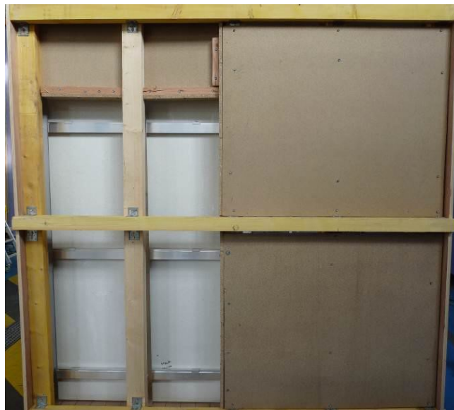
Figure 9: Test assembly with panels and fastenings before the test
