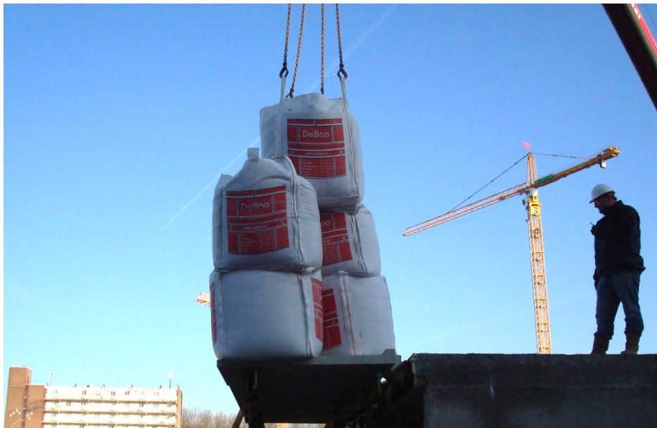
Figure 4: Test loading of a balcony section with 8 \times design load (Poptahof, NL).
