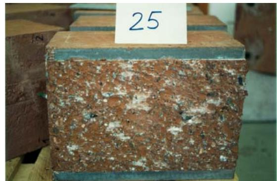
Fig. 3 Fracture faces in test 25 (high-pressure water blasted, 2  $\phi$  12) [3]
