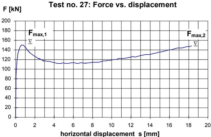
Fig. 2 Load-displacement diagram (high-pressure water blasted, 2  $\phi$  12) [3]
