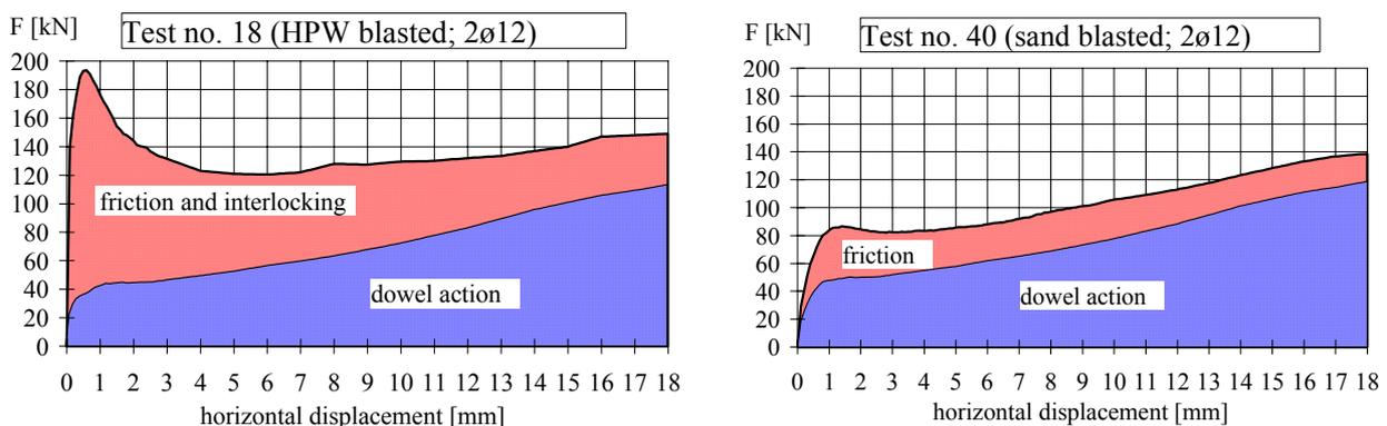
Fig. 5 Components of resistance (high-pressure water blasted and sand-blasted surface)
