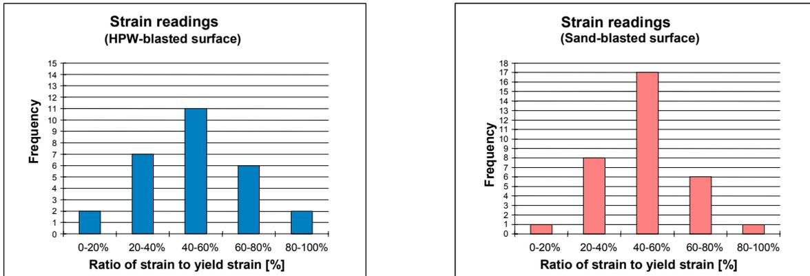
Fig.4 Strain of joint reinforcement (high-pressure water blasted and sand blasted)
