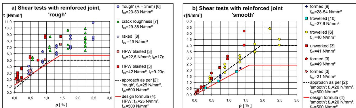
Fig. 6 Comparison of design formula (4) with test results on rough joints (a) and smooth joints (b)
