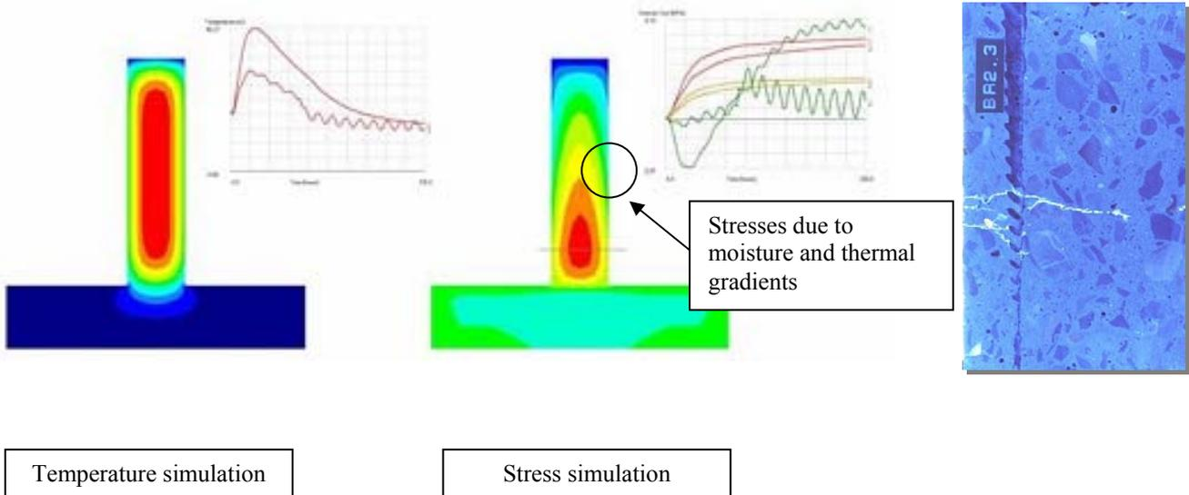
Fig 6. Example of macro-scale simulations [6], Left: Thermal analysis of hardening concrete wall, Right: Thermal crack in concrete, passing the rebar.
