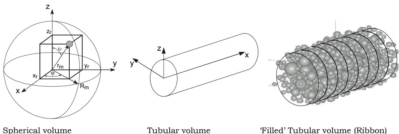
Fig 2. Schematic representation of the confined volumes for random particle structure
