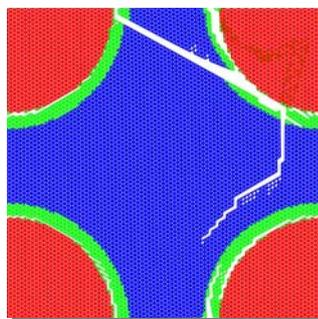
Fig 7. Crack formation calculated with a lattice model at meso-level [6].
