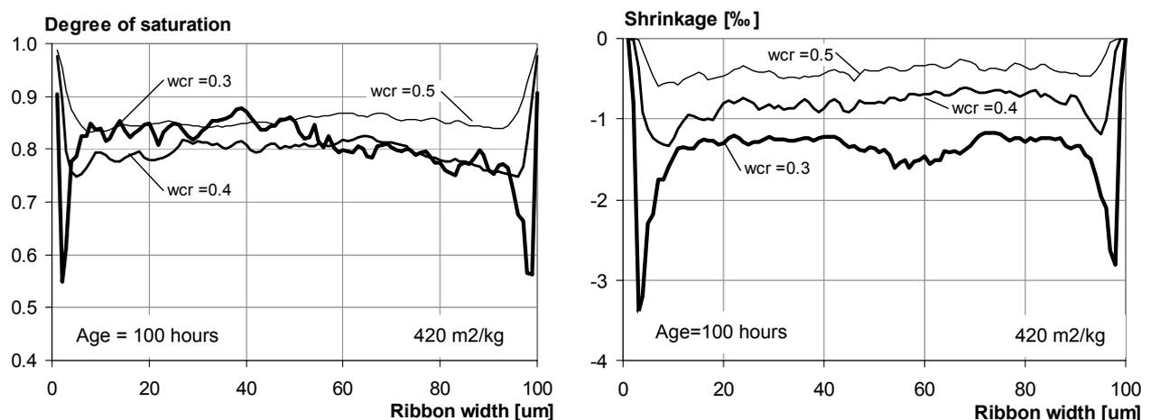
Fig 5. Left: Degree of saturation versus ribbon width, Right: Hardening shrinkage versus ribbon width.
