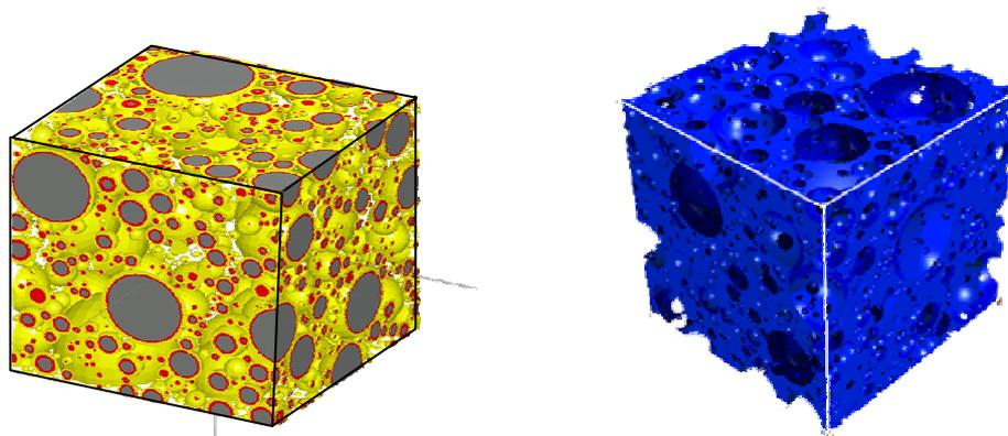
Fig 4. Generated particle structure Left: after hydration, Right: capillary water
