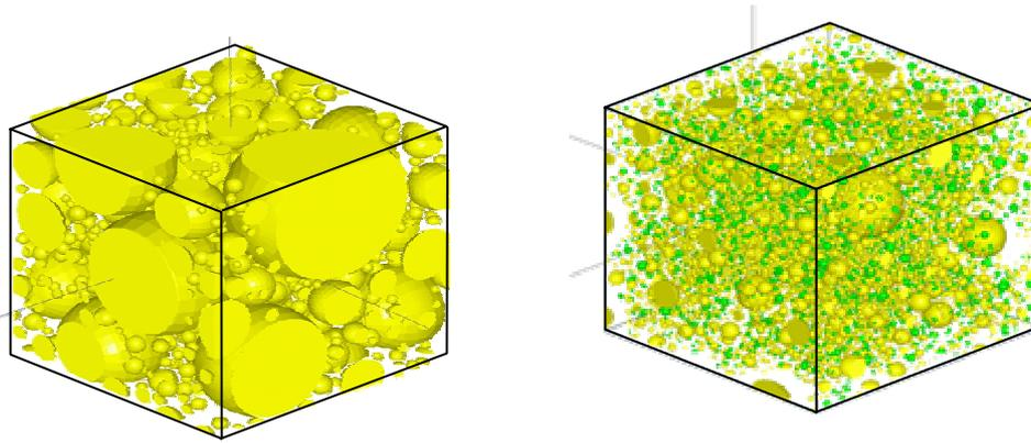
Fig 3. Generated particle structure, Left: cement, Right: cement with fillers.
