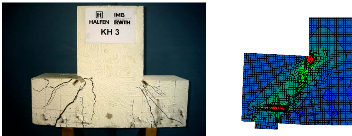
Fig. 4 Test specimen KH 3 and Finite Element Analysis
