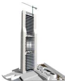
11. The construction of the slabs is finished; the stay's strands are stressed to their final state.
