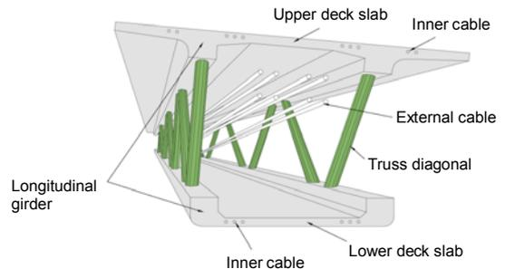
Figure-2. Composite truss bridge
