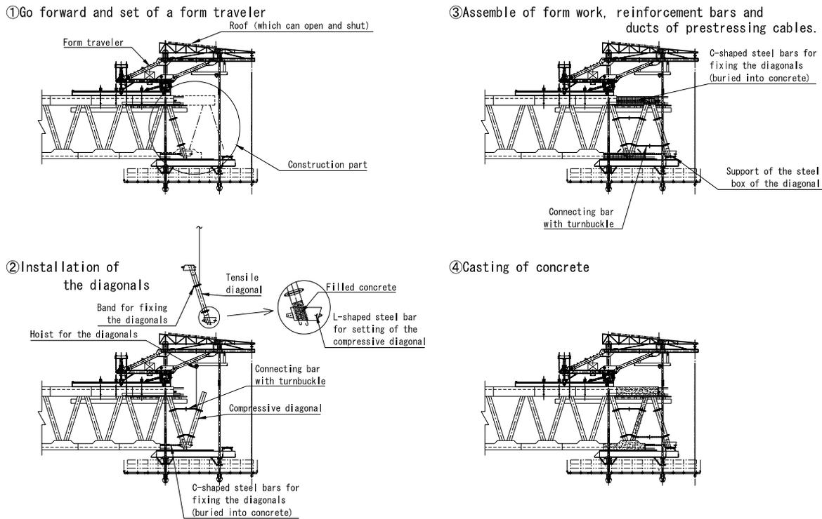
Figure-8. Procedure for cantilevering main girders
