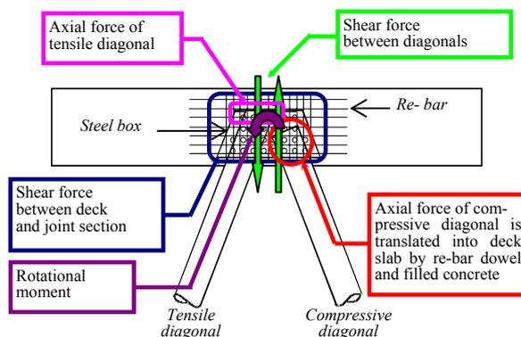
Figure-6. Panel point structure
