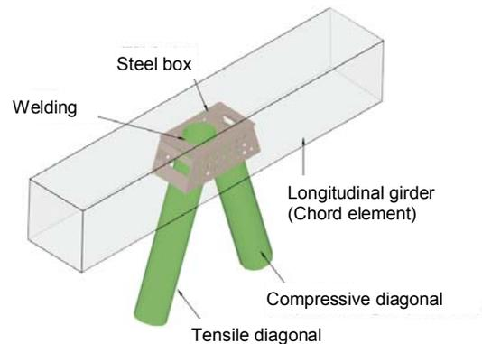
Figure-3. Steel box-type joint
