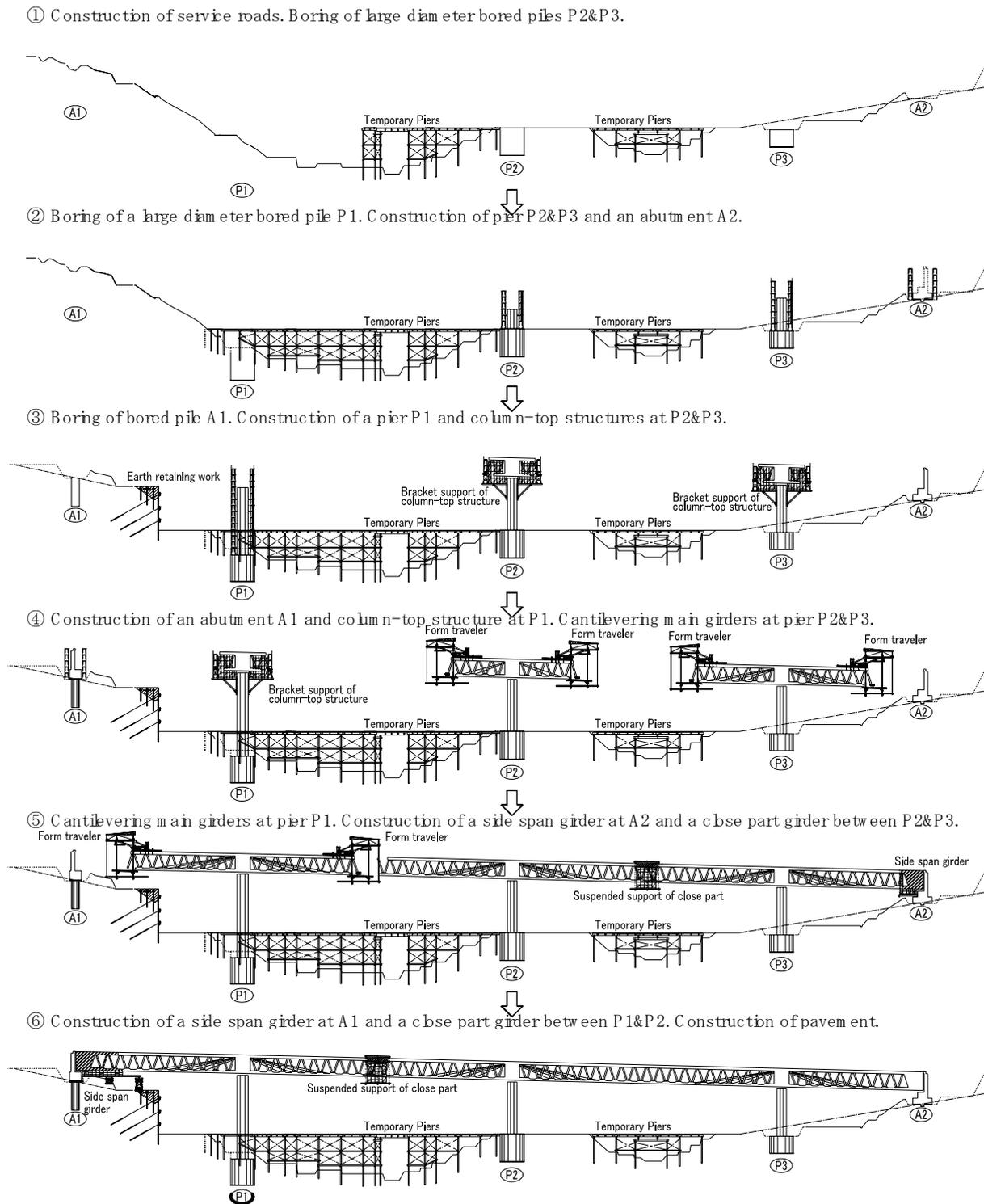
Figure-7. Construction procedure
