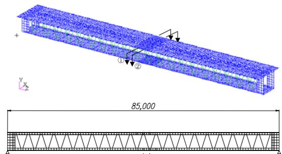
Figure-5. Analysis model of deck slab
