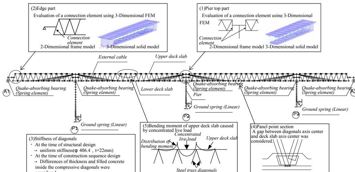
Figure-4. Analysis model of longitudinal design
