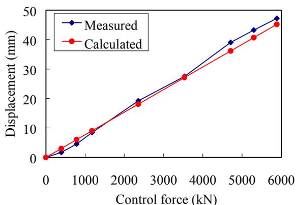
Fig. 8 Comparison of the calculated and measured horizontal displacement
