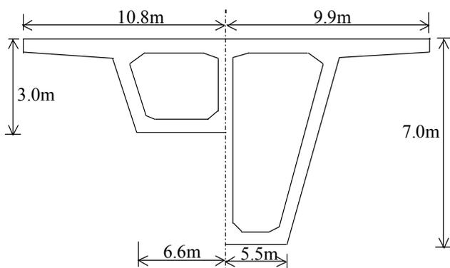
Fig. 4. Cross section
