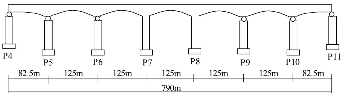
Fig. 3 Elevation of bridge
