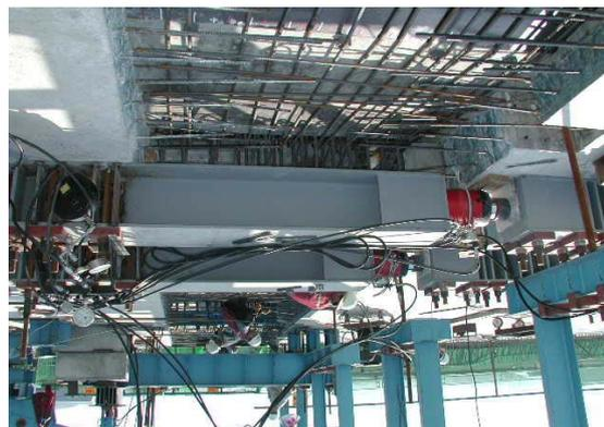
Fig. 5. Equipment of struts and jacking rams
