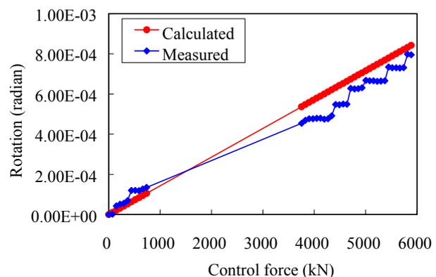
Fig. 9 Comparison of the calculated and measured rotation of the end of pier
