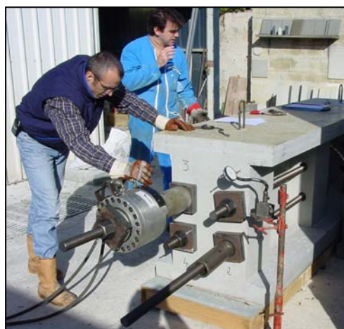
Fig. 12 Bar stitching test by QRD laboratory (Eiffage TP)
