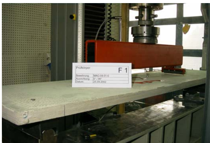
Fig. 9 Four- point- bending test
