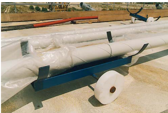
Fig. 5 HDPE duct with helical fillet for stays
