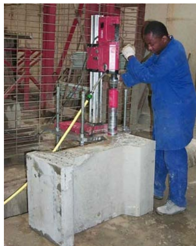
Fig. 3 Drilling of cores in a I beam dummy
