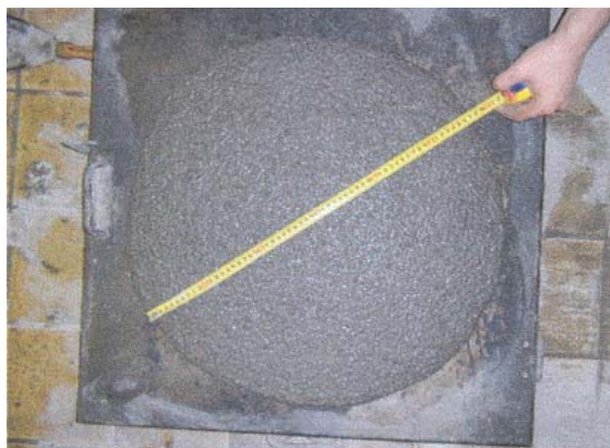
Fig.1. Photograph of consistency by spreading after mixing and after pumping – formula 1.
