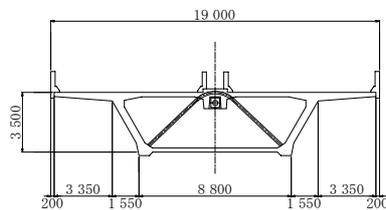
b) Internal struts box - Cross-section area 13.61m<sup>2</sup>
