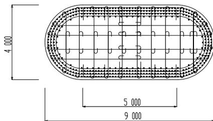
Figure 5 – Pier Cross-Section :
