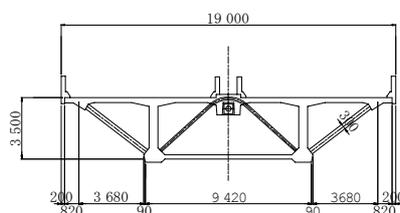
a) Internal and external struts box - Cross-section area 12.62m<sup>2</sup>
