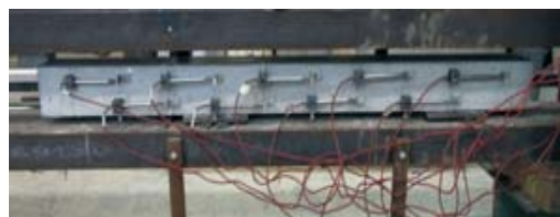
Fig.2 Position of the L.V.D.T (local elongation)
